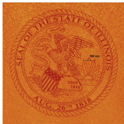
Nanoscale chemical patterns can be made in arbitrary forms. Here, octadecanethiol has been patterned on a gold substrate using dip-pen nanolithography. Image courtesy Andrew Senesi and Chad Mirkin, Northwestern University.
